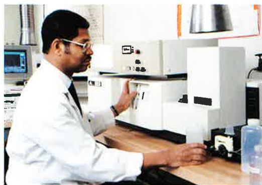
Many elements can be identified on the Direct Current Plasma Spectrometer. This test provides quantitative and qualitative data on trace element impurities in the ppm to ppb range.
