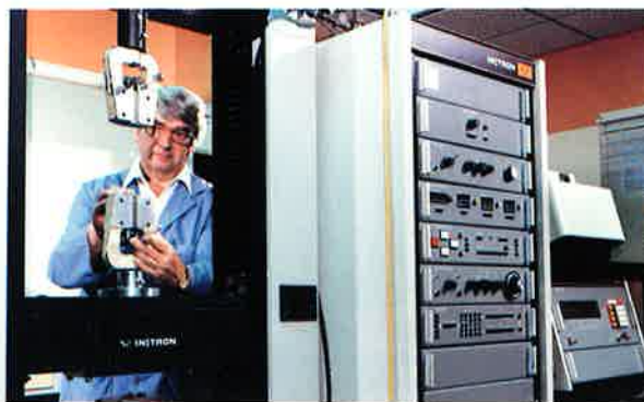
Mechanical properties of tungsten wire are obtained by testing representative samples in tension and/or compression at temperatures from ambient to 2200°C on the Instron Universal Tester.
