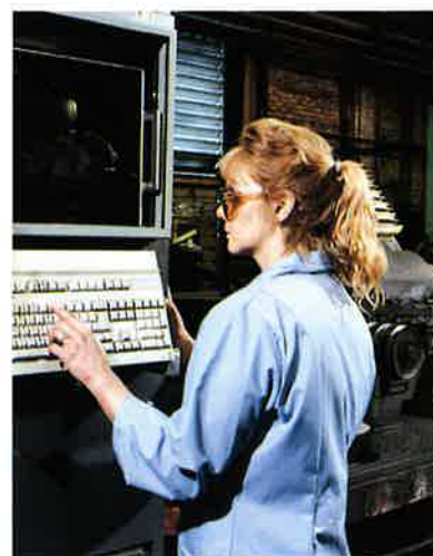
Split levels in tungsten wire are continually monitored as the wire is drawn through a multiple series of dies.
