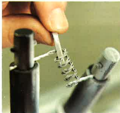
In the vacuum chamber, metal clips to be vaporized are inserted into tungsten metallizing coils.
