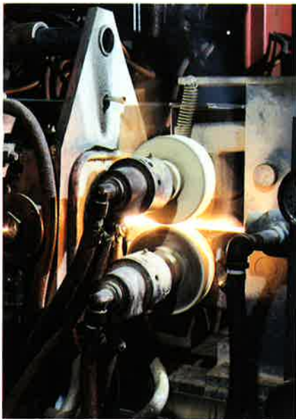
Tungsten rod is processed through a high temperature induction furnace to create a crystal structure with the properties needed for downstream wire drawing operations.
