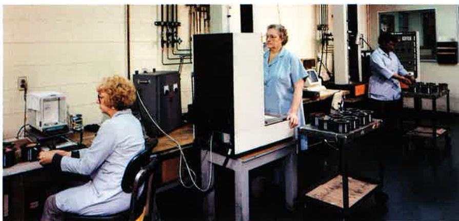
In our quality control lab on the manufacturing floor, samples taken from actual production runs are tested for hot and cold tensile strength, camber, roundness, diameter and other characteristics.
