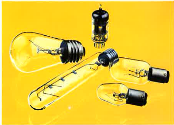
The addition of 3% rhenium to tungsten creates a wire that resists the vibration that occurs in such applications as vacuum cleaner, refrigerator, and aircraft lamp filaments.
