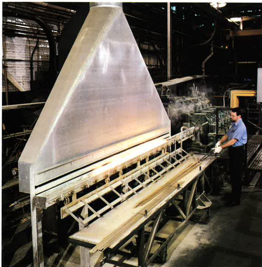
Tungsten rod preheated to 1500°C is passed through multistand rolling mills for reduction to the desired rod diameters.
